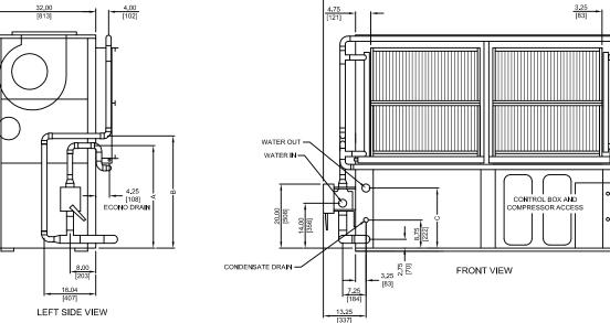
Fig. 12 — 50BVC, J, Q020-028 with Optional Waterside Economizer Dimensions
